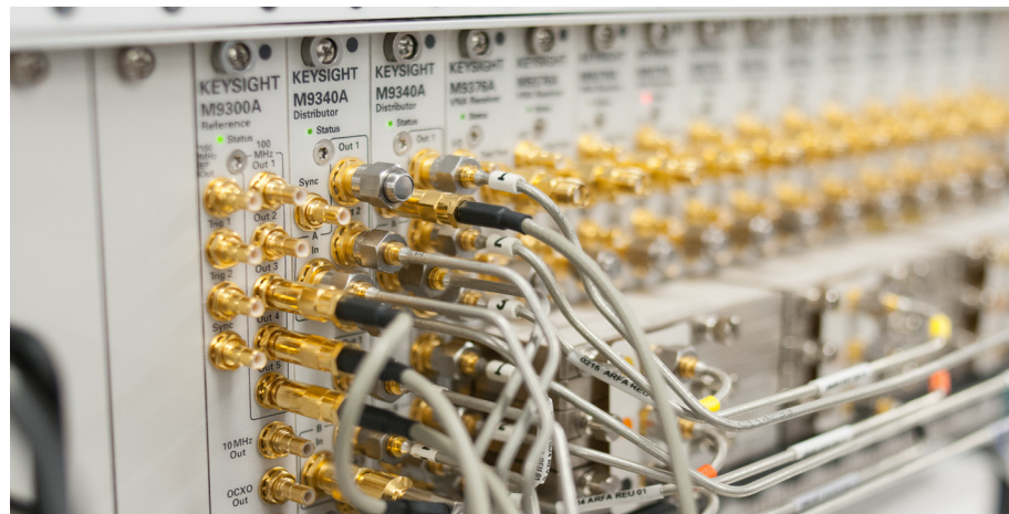
Figure 3. New M9485A multi-port VNA.
