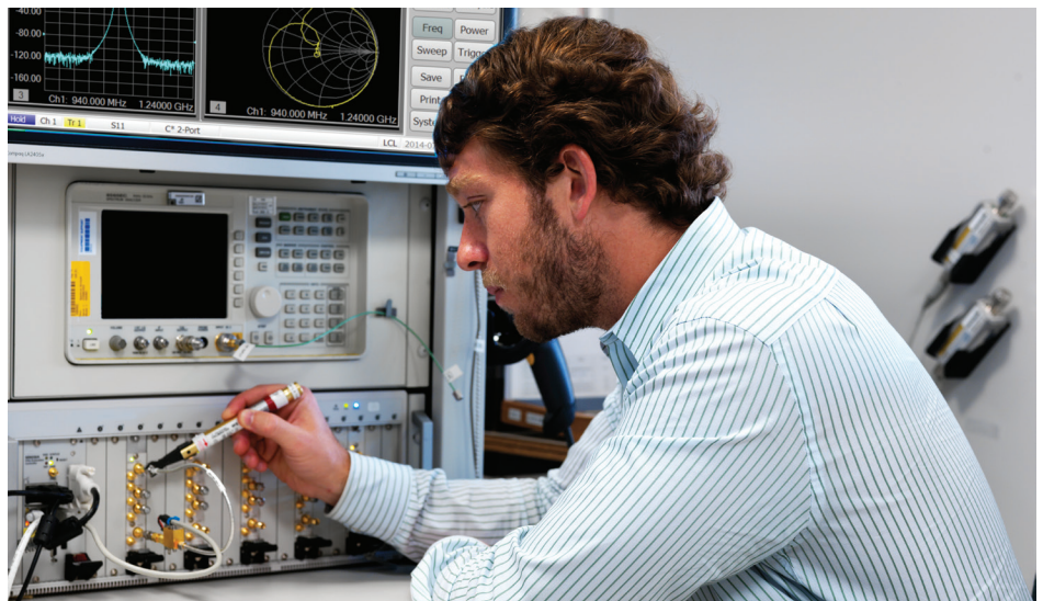
Figure 1. Adding a pair of 2-port PXI VNAs to an existing test station enables powerful device characterization without expanding system height or footprint.
